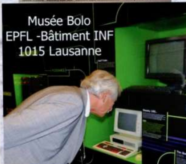
Smaky Microcomputer, Epitac Systems, Switzerland, 1978 The Smaky Microcomputer was designed by the Smaky, or Smart Keyboard, as a teaching computer. It was part of a classroom network with a Data Central Host as a server. Speed: 0.2MHz Memory size: 32K Memory type: Random Access Memory width: 8-bit
