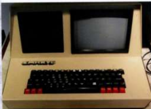
Smaky Microcomputer, Epitac Systems, Switzerland, 1978 The Smaky Microcomputer was designed by the Smaky, or Smart Keyboard, as a teaching computer. It was part of a classroom network with a Data Central Host as a server. Speed: 0.2MHz Memory size: 32K Memory type: Random Access Memory width: 8-bit
