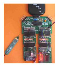
Microdules are a set of cards, a kind of meccano, that allows to change easily the processor and the interface modules to configure any application with a minimum of special wiring. The objective is to develop the hardware and software in an environnement where it is easy to adapt to the needs of changing the hardware and adding debugging helps.
