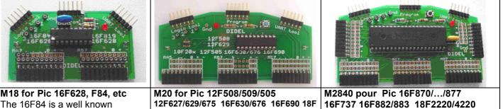
The 16F84 is a well known controller with powerful successors, on which Analogue inputs, Uart, I2C, PWM are available.
