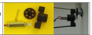
For 6mm pagers, the gearbox includes a propsaver connector. Ratio is 5.3 . Weight witout motor and propeller 0.53g
