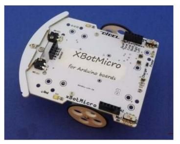
XBotMicro swiss design is a small, low power robot base, with all what you need to test sensors and behaviours and learn a lot about C programming and robots. During software development, it is powered by the microcontroller card 5V, 100mA. Autonomous operations are powered by its included rechargeble battery 3.2 to 3.7V 150mAh.
