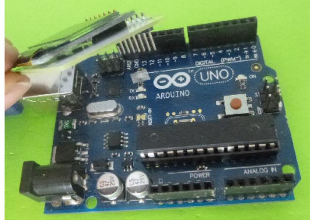
Oled module SSD1306 on Didel adapter and inserted on top left Arduino connector
