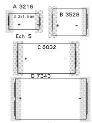
Normal capacitors have 2 pins with a spacing of 2.5 mm (sometimes 5mm) up to 10 microfarad. SMD capacitors starts with the same sizes as SMD resistors: 0402, 0603,
