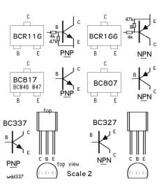
Transistors are only considered here as switching devices. They should be saturated or open.
