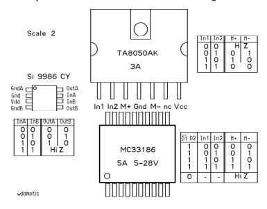
For the best control, the motor must be breaked (short circuit), but this increases significantly the power consumption. A PWM control with ON/High-Z state consumes much less current
