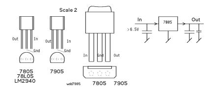
Low drop-out regulators have a lower voltage drop. This means they can provide 5V from 5.6V, and heat less for voltage drop of e.g. 3V. A diode between the gnd pin and ground will change the output voltage by 0.6~V~(1N914) or 0.3V~(BAT42) if one need 5.6~or~5.3V.
