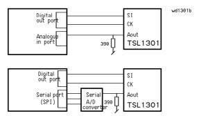
A microcontroller program will prepare a pointer in memory, generate the clock and store the data in memory. Processing for defining the shape and position of objects may be done while acquiring the pixels, or on the values stored in memory. The most efficient is to do it real time and not store the complete image, but frequently a combination of both is required.
