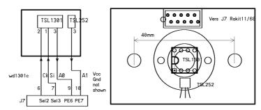
A first HC11 test program (Test 28 on Rok11c2), intended to check the correct operation with an oscilloscope, and adjust the focus, is given below. A sheet of black paper with a one cm wide slot, lighted from behind, is used to adjust the focus.
