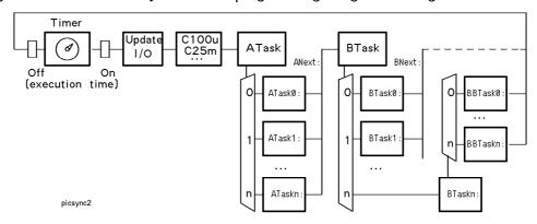
The timer synchronizes on a fixed period basis. There should be some waiting time before resynchronisation: the best way to measure it is to clear a free bit on a port before starting the wait for the timer and set it when the timer is reinitialized. A scope will clearly show the execution time every 100  $\mu$ s. There will be an important jitter if the subtasks are not of similar length. If the time is too long, the time will miss one turn, and this is easy to recognize on the scope.
