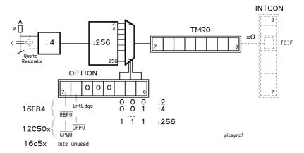
The processor clock (quartz or RC network) is divided by 4 to give the 1 MHz frequency that defines the 1 microsecond instruction time that will always be our reference. A programmable predivider is implemented before the TMRO counter that can be read and written by the processor.
